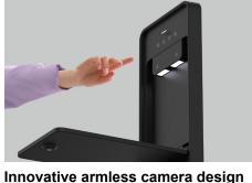
The innovative armless camera with tilt-shooting technology ensures the quality and efficiency of your performance. High-brightness LED lighting ensures even illumination of documents.
